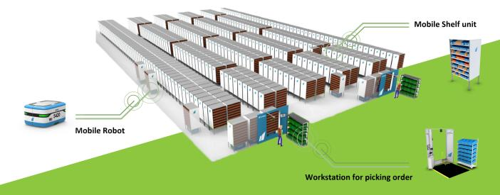
The use of ultra-modern, automated storage and retrieval systems (Automated Storage and Retrieval System / ASRS) ensures a future-oriented logistics concept.
