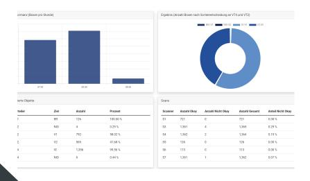
The XPROMA WCS also includes customized visualization and reporting of the automated line. This means that the status of the conveyor technology, machine or peripherals can be called up and viewed by the customer on any PC.
