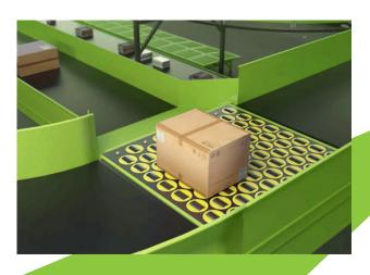
As a stand-alone module, the Pivot Wheel Sorter can be used in combination with conveyors and can be deployed anywhere at the conveyor line.
